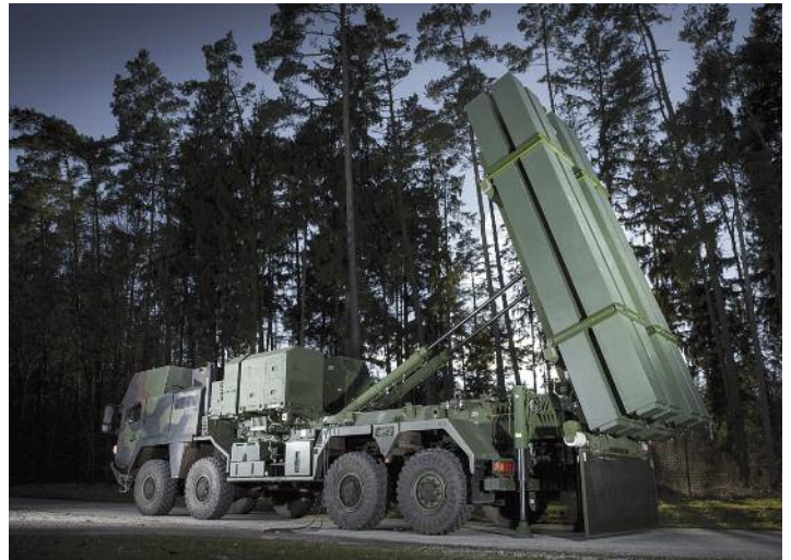
A lightweight MEADS launcher in the German configuration is A400M transportable and can engage and defeat targets attacking from any direction.
